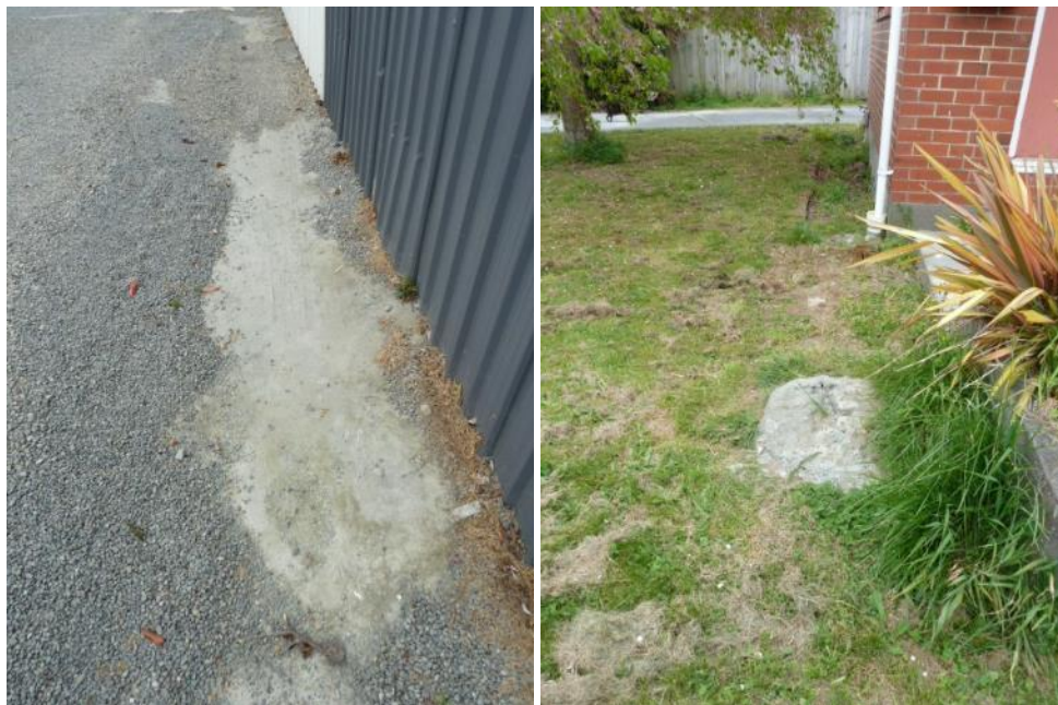
Figure 38: Ground photograph showing ejecta at a nearby property (49 and 49A Halswell Rd).
